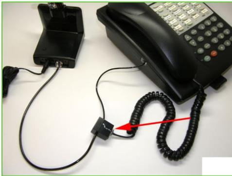
Plug your telephone handset cord into the middle of the Telephone Interface Cable (black box).
